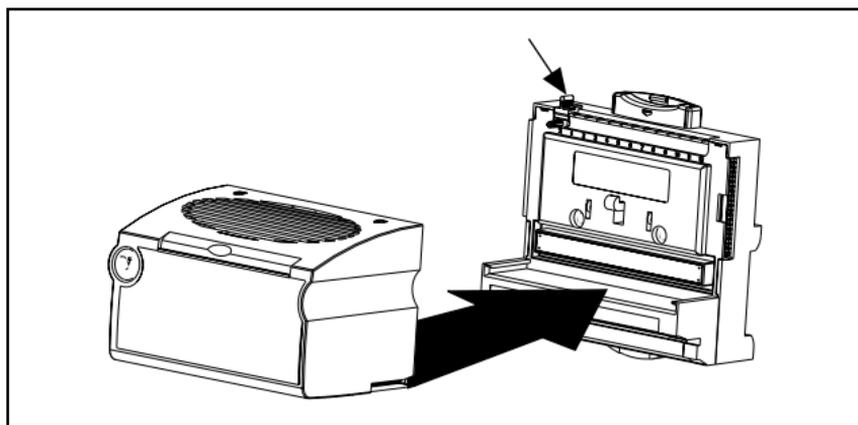
2. Position the I/O module with its alignment slots aligned with the guide rails on the terminal base.
