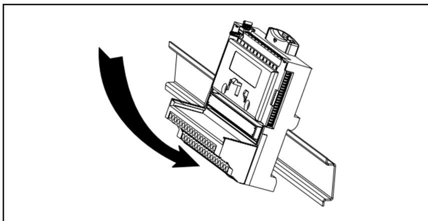
3. Slide the terminal base along the DIN rail until its local bus connector mates with the connector of the terminal base or network module adjacent to it.
